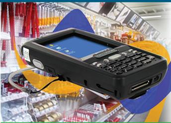
The rugged PHL 8112 PDA features an integrated 1D scan engine and a full color 3.5" TFT display, with a numeric (dial) keypad. This product is Bluetooth & WiFi interfaced and Cisco CCX compliant for data capture in mobile business.
